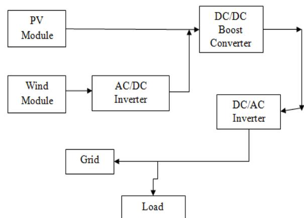
Figure 2: Hybrid energy system topology
