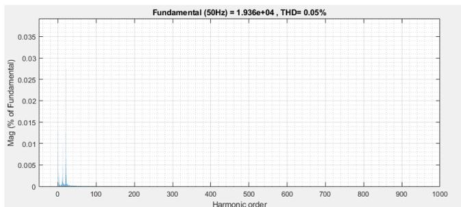
Figure 12: THD% of Voltage output from the system with Compensator having voltage regulation by linear crow search optimization (VL-CSA)
