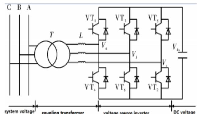
Figure 1: Basic Structure of STATCOM
