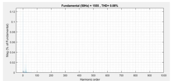
Figure 14: THD% of Current output from the system with Compensator having voltage regulation by linear crow search optimization (VL-CSA)
