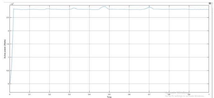
Figure 9: Active Power output from the system with STATCOM having Vdc / Vac control using PI controller
