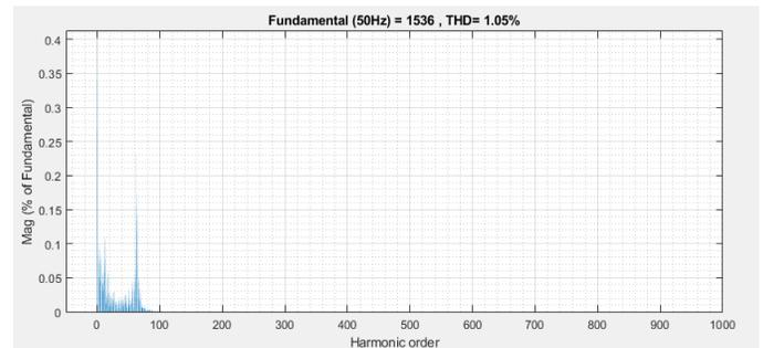
Figure 8: THD% in Current output from the system with STATCOM having Vdc / Vac control using PI controller
