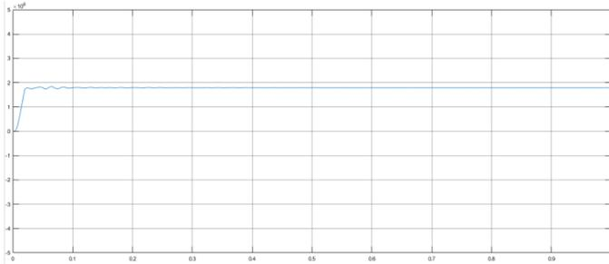
Figure 16: Reactive power output from the system with Compensator having voltage regulation by linear crow search optimization (VL-CSA)
