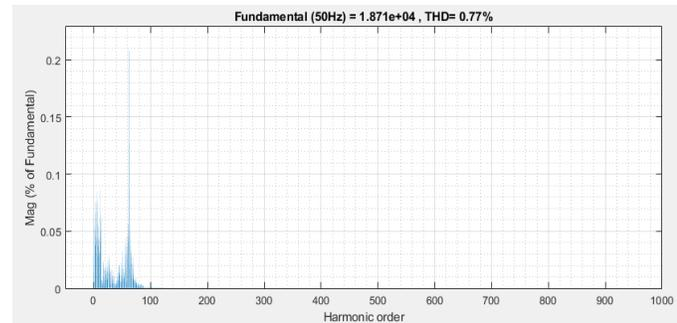
Figure 6: THD % Voltage output from the system with STATCOM having Vdc / Vac control using PI controller
