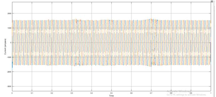
Figure 7: Current output from the system with STATCOM having Vdc / Vac control using PI controller
