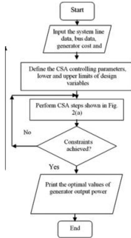
Figure 4: Designing of proposed methodology for compensation in large scale renewable energy resources
