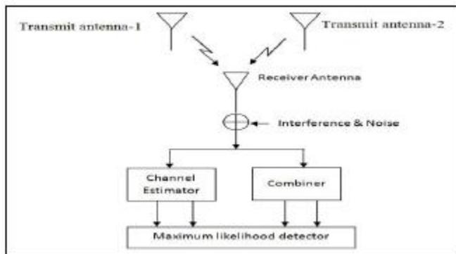
Fig1: Generalized system model used for simple transmit diversity technique
