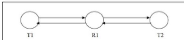
Fig5. Two-Way Relaying network
