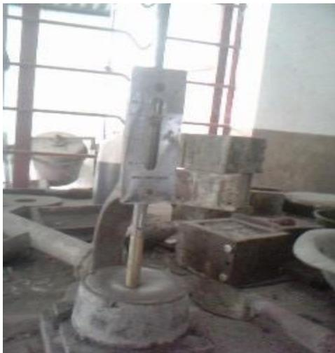
Fig 3.1 Vicat Apparatus for Normal consistency
