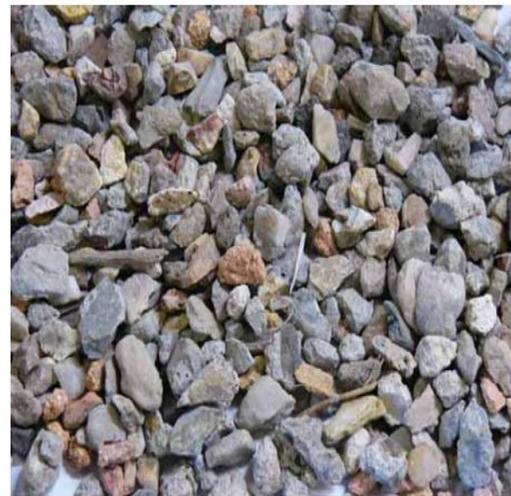
Figure 1.1: Recycled Aggregate
