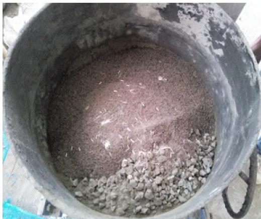
**Figure 3.2** Mixing of glass fibres, Cement, coarse & fine aggregate
