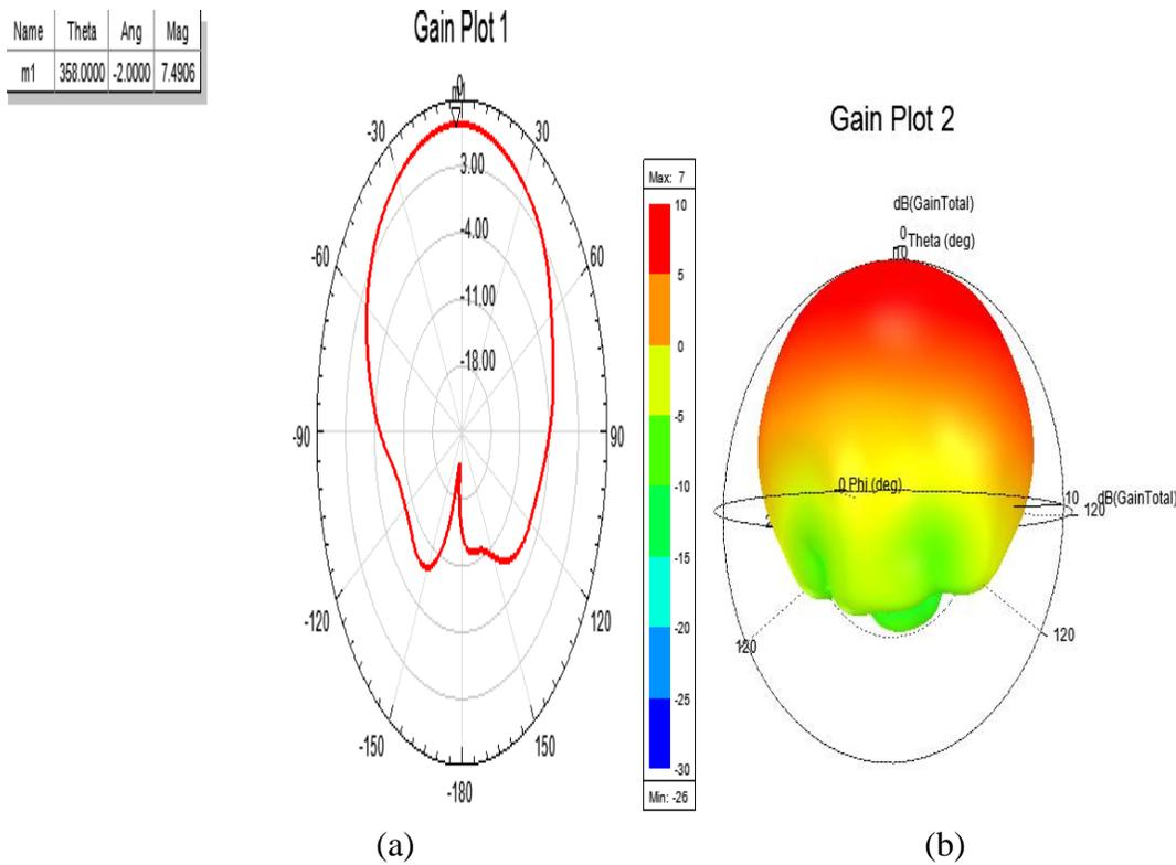
Fig. 3. 2D and 3D gain representation of the microstrip patch antenna
