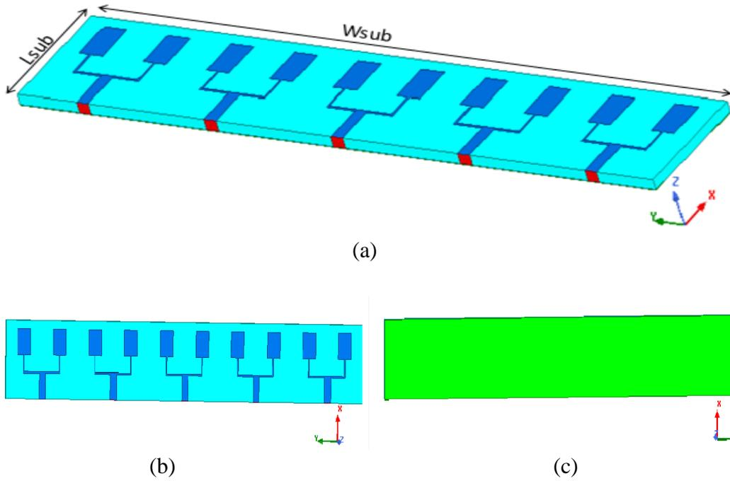
Fig. 4. Design of proposed 5G antenna array with five sources (a) Side (b) Top and (c) Bottom views
