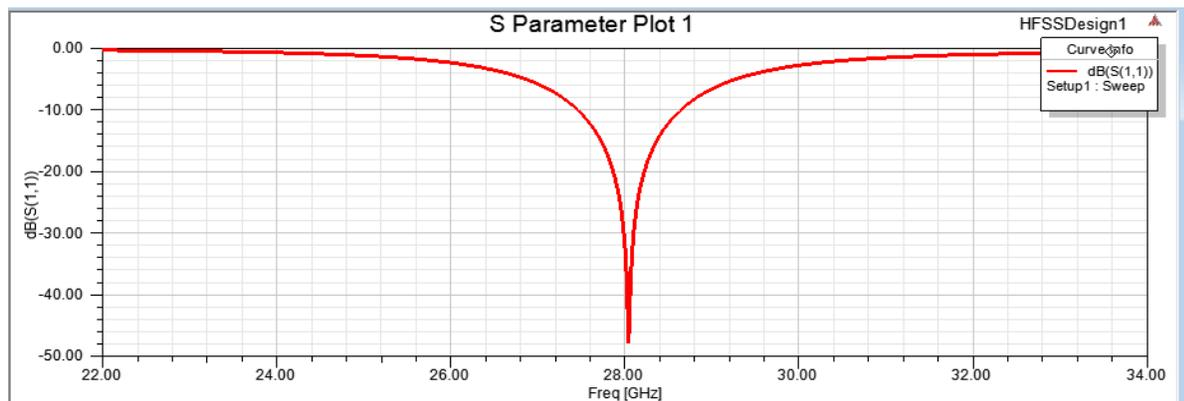
Fig. 2. Simulated S-parameter of the microstrip patch antenna
