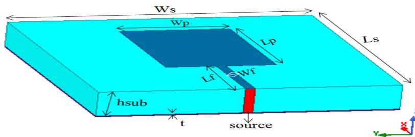
Fig. 1. Design of Single patch antenna
