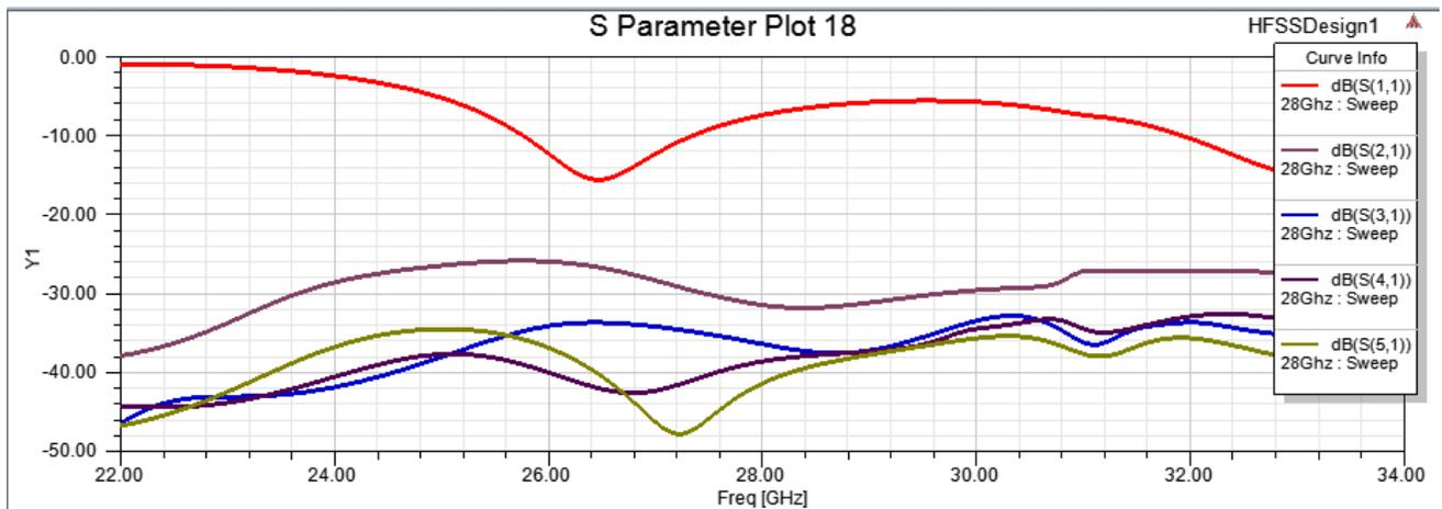
Fig. 5. S-parameters of the proposed antenna array
