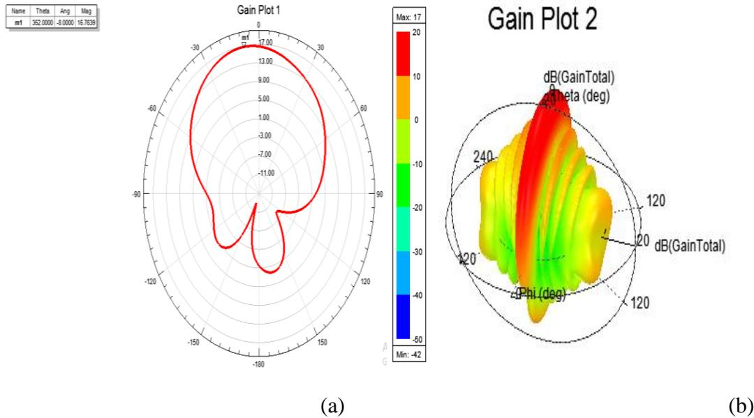
Fig. 6. (a)2D, (b)3D gain plot of the proposed antenna array
