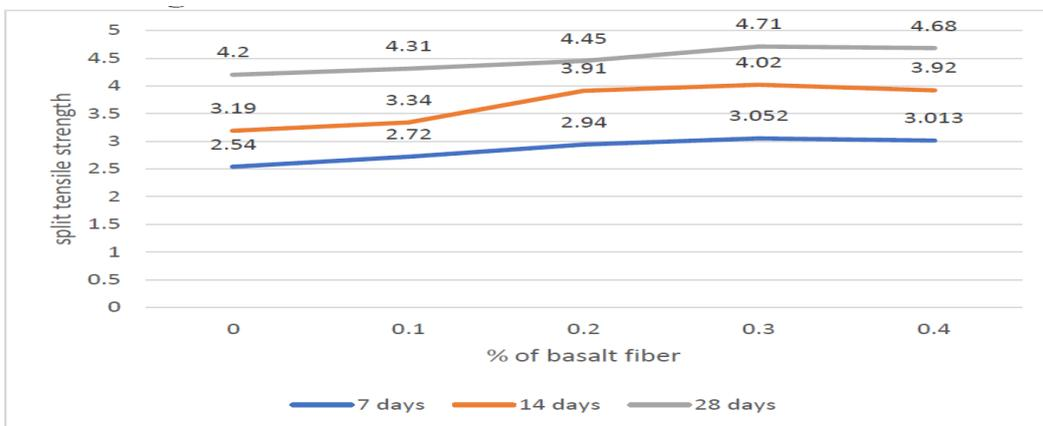
Figure 13: Graph of split tensile Strength comparison at 7, 14 and 28 days for M30 concrete
