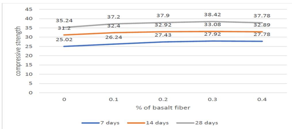
Figure 11: Graph of Compressive Strength comparison at 7, 14 and 28 days for M30 concrete
