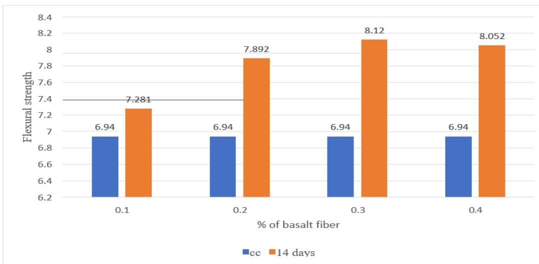
**Figure 8: Comparison of flexural strength of M30 concrete at 14 days**
