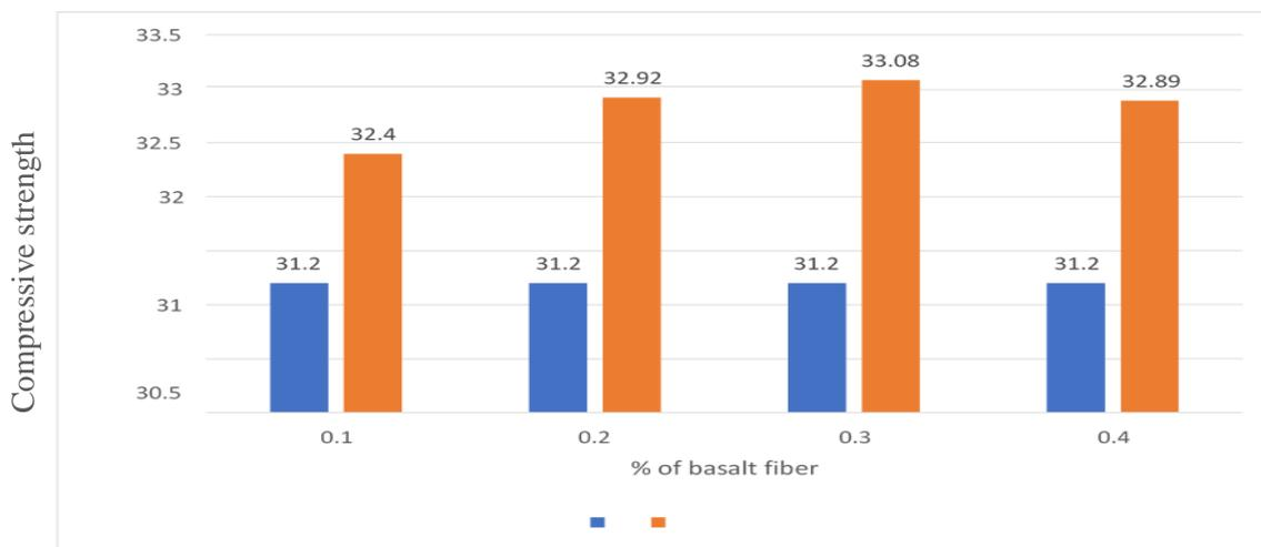
Figure 2: Comparison of Compressive strength of M30 at 14 days
