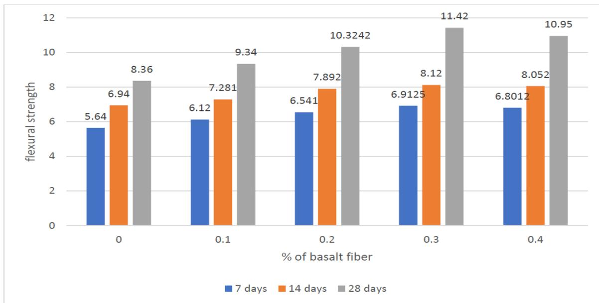
**Figure 16: Flexural Strength comparison at 7, 14 and 28 days for M30 concrete**
