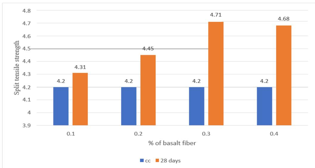
Figure 6: Comparison of Split tensile strength of M30 at 28days
