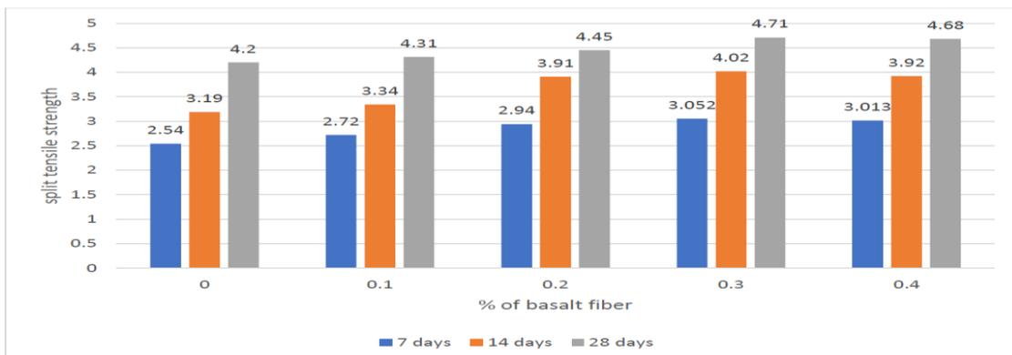
Figure 14: Split tensile Strength comparison at 7, 14 and 28 days for M30 concrete
