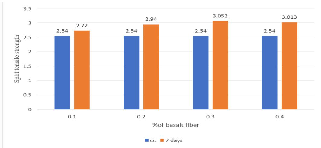
Figure 4: Comparison of Split tensile strength of M30 at 7days
