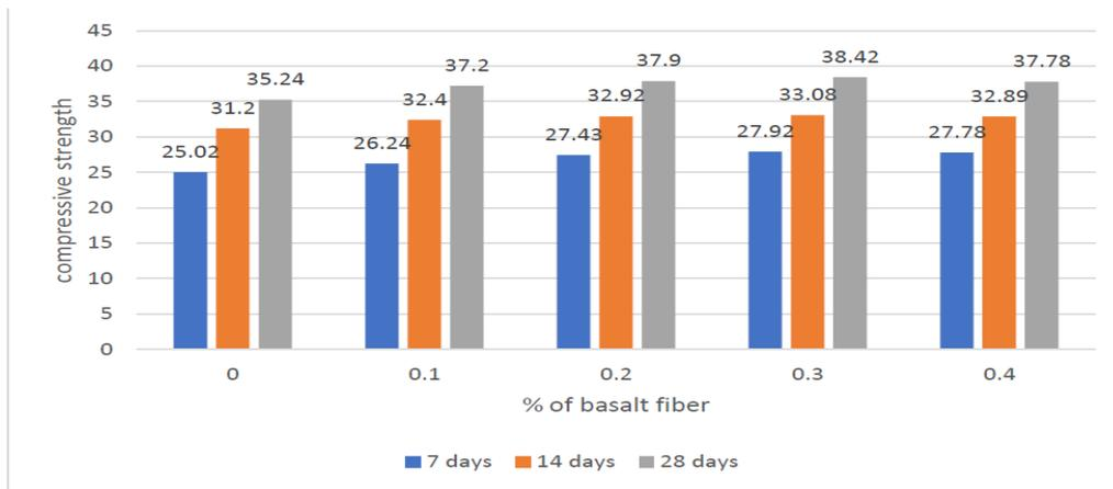
Figure 12: Compressive Strength comparison at 7, 14 and 28 days for M30 concrete
