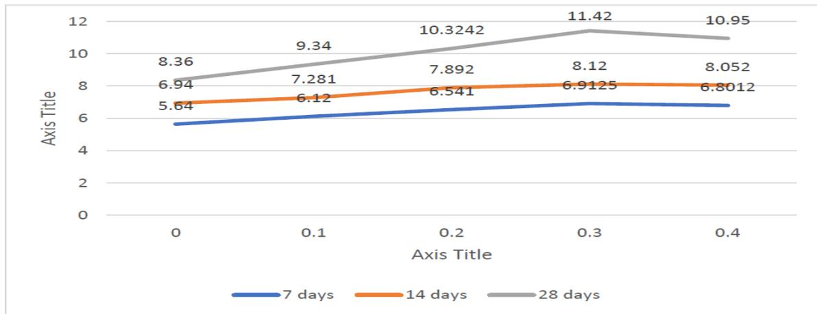
**Figure 15: Graph of flexural Strength comparison at 7, 14 and 28 days for M30 concrete**
