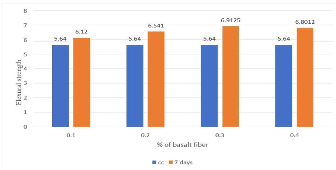
**Figure 7: Comparison of flexural strength of M30 concrete at 7 days**
