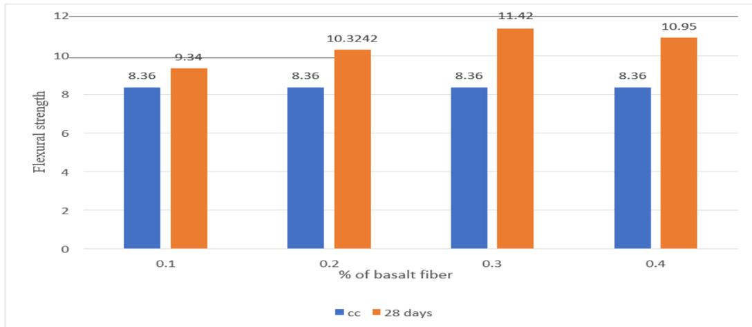
Figure 9: Comparison of flexural strength of M30 concrete at 28 days
