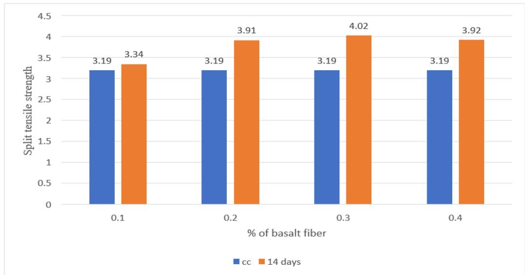
Figure 5: Comparison of Split tensile strength of M30 at 14days
