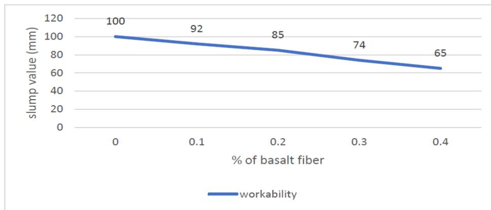
Figure 10: Comparison of workability for different mixes of M30 Grade
