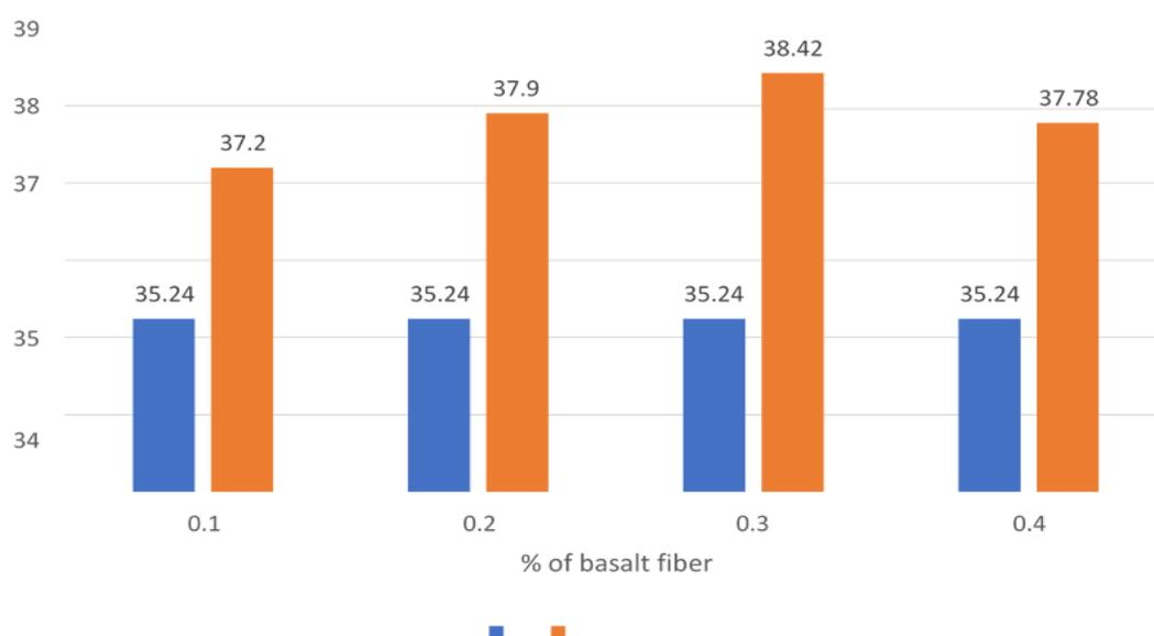
Figure 3: Comparison of Compressive strength of M30 at 28 days
